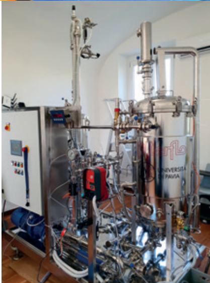
Experimental device built by the University of Pavia to extract bioethanol from waste materials
